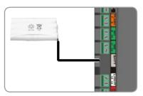
Connect the battery to the electronic module terminal provided for this purpose (grey label "BATT").
